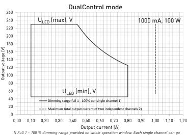
down to 1 % dimming at 100 - 800 mA.
