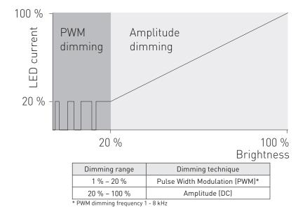
Helvar hybrid dimming products combine the best features from Amplitude dimming and from Pulse Width Modulation (PWM) dimming. CCR is a very efficient technique for dimming the light output especially on higher range. On lower range, the hybrid dimming products implement high-frequency PWM dimming to ensure high quality dimming from 20 % down to 1 % providing low flicker dimming performance.
