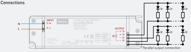
Attention: If using LL1-CV-DA or LL1-CV-SC control units to control LED load with this driver, make sure the total output current from the LL1x75-CV12 driver does not exceed 5 A (60 W)!
