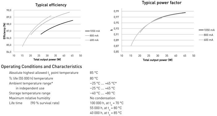
\*) For other than independent use, higher t, of the controlgear possible as long as highest allowed t, point temperature is not exceeded
