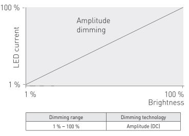
LL165HE-DA-300-1050-IND LED driver implements amplitude dimming technology across whole dimming range. Amplitude dimming offers the best available technology for dimming the light output in an accurate and flicker-free way to ensure high quality lighting in even the most demanding situations such as camera recording applications. Amplitude dimming technology complies with IEEE 1789-2015 recommendations of current modulation to mitigate health risks to viewers.
