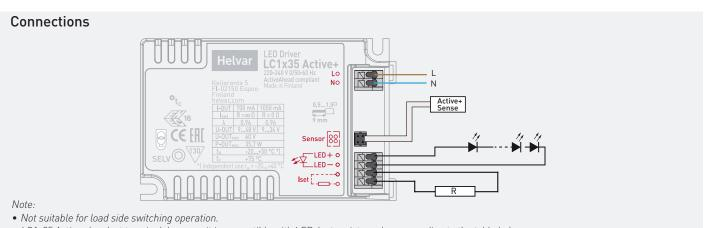
• LC1x35 Active+ has Iset terminal, however it is compatible with LED-Iset resistor values according to the table below.
