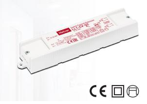
The LL1-CV-SC Switch-Control dimmable extension unit is designed to be used with the Helvar constant voltage LED drivers, creating controllable solutions for decorative lighting. It enables the use of Helvar Switch-Control, which is a protocol for controlling the light with a retractable switch, in constant voltage (12 - 24 V) lighting applications.
