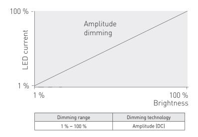
LC51SE-DA-900-1400-LOOP LED driver implements amplitude dimming technology across whole dimming range. Amplitude dimming offers the best available technology for dimming the light output in an accurate and flicker-free way to ensure high quality lighting in even the most demanding situations such as camera recording applications. Amplitude dimming technology complies with IEEE 1789-2015 recommendations of current modulation to mitigate health risks to viewers.
