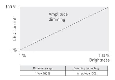
LC45SE-DA-600-1050-LOOP LED driver implements amplitude dimming technology across whole dimming range. Amplitude dimming offers the best available technology for dimming the light output in an accurate and flicker-free way to ensure high quality lighting in even the most demanding situations such as camera recording applications. Amplitude dimming technology complies with IEEE 1789-2015 recommendations of current modulation to mitigate health risks to viewers.
