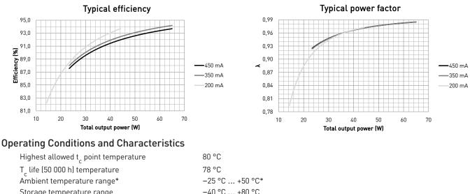
Storage temperature range Maximum relative humidity Lifetime (90 % survival rate) -40 °C ... +80 °C No condensation 100 000 h, at t = 65 °C 70 000 h, at t<sub>c</sub> = 70 °C 50 000 h, at t = 78 °C 35 000 h, at t = 80 °C
