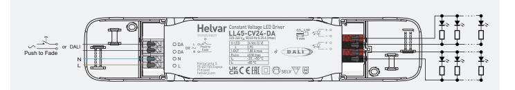
Note: Avoid using longer LED strips that 5 meters, the voltage losses grow substantial with long runs. In case of uneven brightness of LEDs in long strips, parallel connection of shorter strips is recommended.
